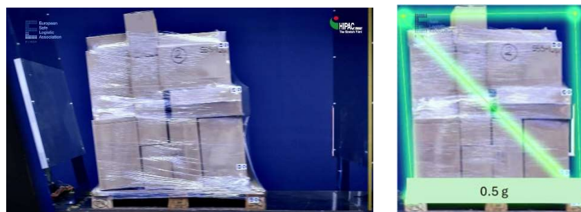
Fig. 5. EUMOS 40509-20 Test pallet stability
